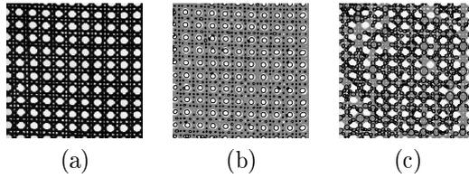
Figure 6: *BD* of original image in (a). Bright blobs are represented in (b) and dark ones in (c)
