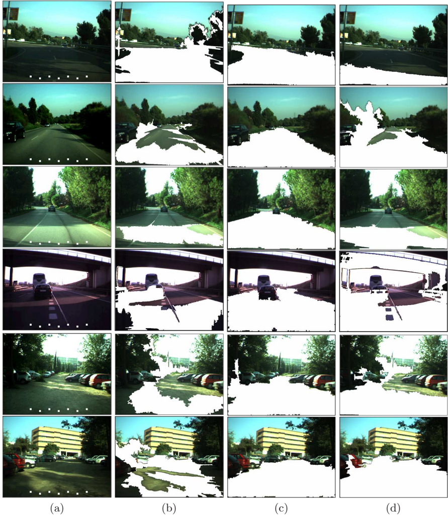
Fig. 4. From left to right columns: (a) original 640 \times 480 color image with the seven used seeds marked in white; (b) segmentation using I with t_{agg,I} = 0,008 ; (c) segmentation using I with t_{agg,I} = 0,003 ; (d) segmentation using HSI with t_{agg,ch} = 0,08 , and t_{agg,ach} = 0,008 . The white pixels over the original image correspond to the segmentation results. The top four rows correspond to asphalted roads and the rest to non-asphalted areas of a parking.
