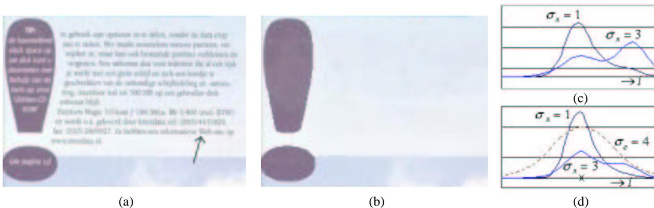
**Fig. 2.** a) input image (230x160) b) global mode of input image with  $\sigma_x = 3, \sigma_i = 16$  and  $\beta = 16$  c) local histogram at two scales (projected with  $i = R + G + B$  for visualisation purposes) of character in input image,  $\sigma_i = 8$ , location character is indicated with arrow. d) constraint mode with  $\sigma_c = 4$  of histogram of c).
