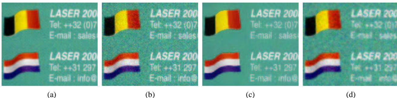
**Fig. 3.** a) input image (150x130) b) corrupted with uncorrelated Gaussian noise  $\sigma = 20$  c) constrained mode with  $\sigma_x = 4, \sigma_i = 48, \sigma_c = 1.75$  and  $\beta = 16$  d) vector median (3x3 neighborhood) as proposed in [1]
